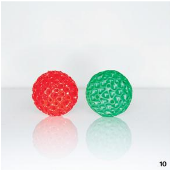
10–11 The printers can also build objects from bouncy, flexible elastomers, which could be well suited for wearable items like shoe soles and headphones. Elastomers are incompatible with traditional additive manufacturing, says DeSimone.
