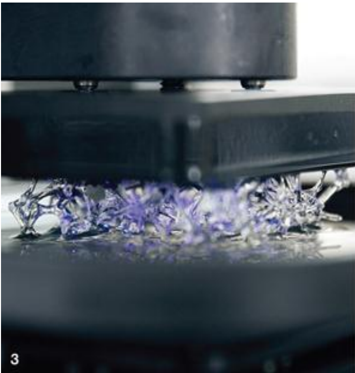
2-4. Frame by frame, the ultraviolet light projects the design into the chemical bath. Some of the light is visible as a violet glow
