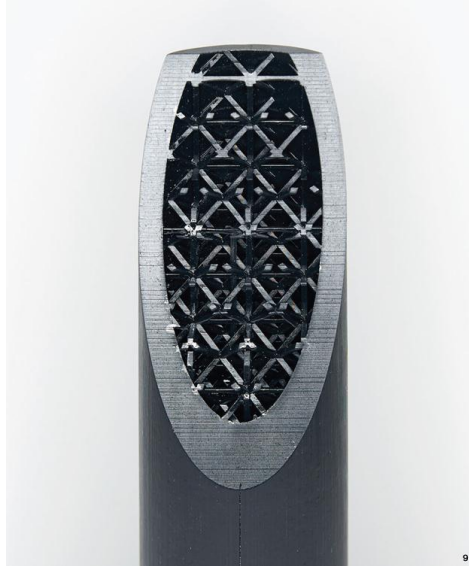
9. A pattern of struts inside this 3-D-printed cylinder of hard resin adds extra strength without adding much weight. This kind of design might be used to replace metal support structures in airplane seats, according to the company.
